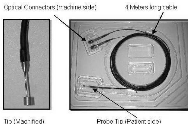
**Fig. 6:** The TSP2000-2 probe for brain cortex monitoring
