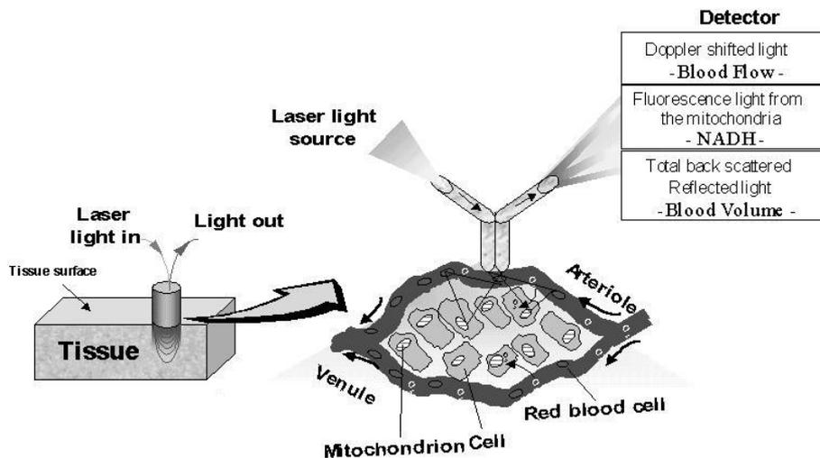
**Fig. 2:** The technical principles of the TiSpec. A single light source was used and the emitted light from the tissue is collected by optical fiber to the detection system.
