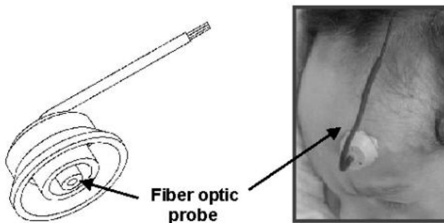
**Fig. 8:** The TSP-NB1 Neonates monitoring probe (Left) attached to a baby's forehead skin (right)
